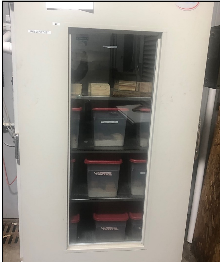
Figure 2.2 Testing containers incubated in climate-controlled incubation chambers set at 70°F with 64% RH and 12% EMC.
