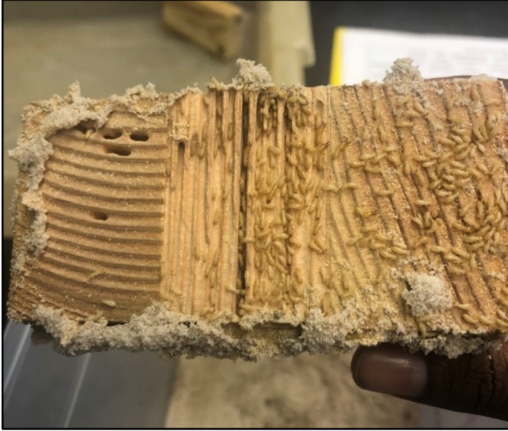
Figure 4.4 CLT HF specimen with active termites attacking between narrow and wide growth rings.
