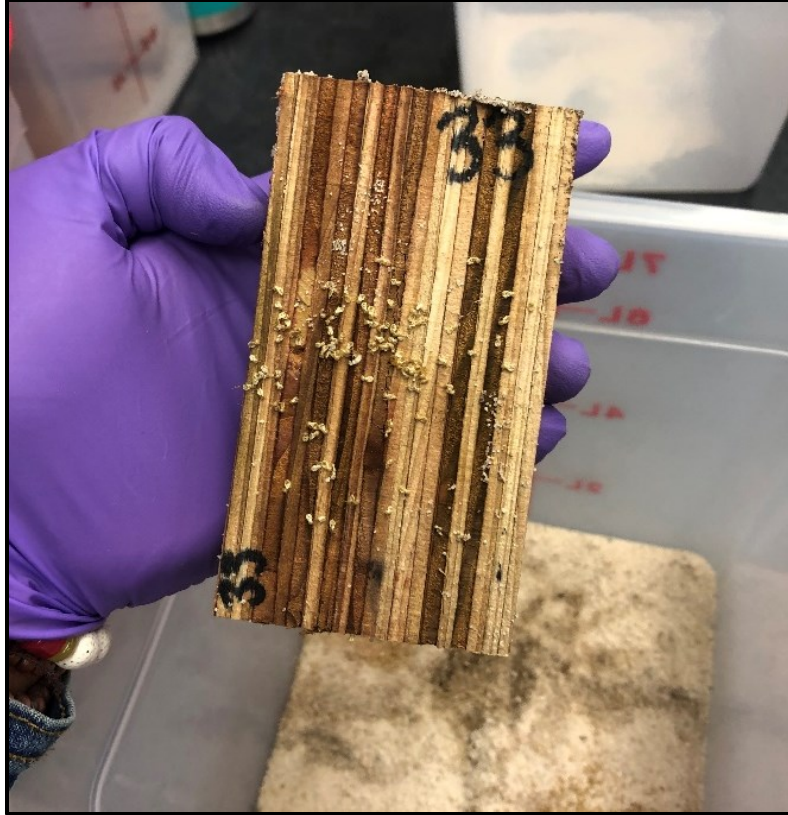
Figure 4.1 MPP sample #33 of Treatment D (MPP paired with Hem-Fir CLT) with dried termites on the exposed surface.
