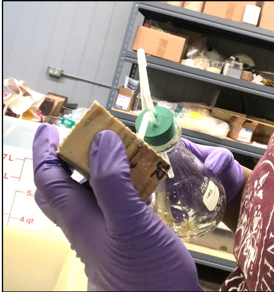
Figure 2.3 Removal and counting of termites at the end of testing using a vacuum aspirator.
