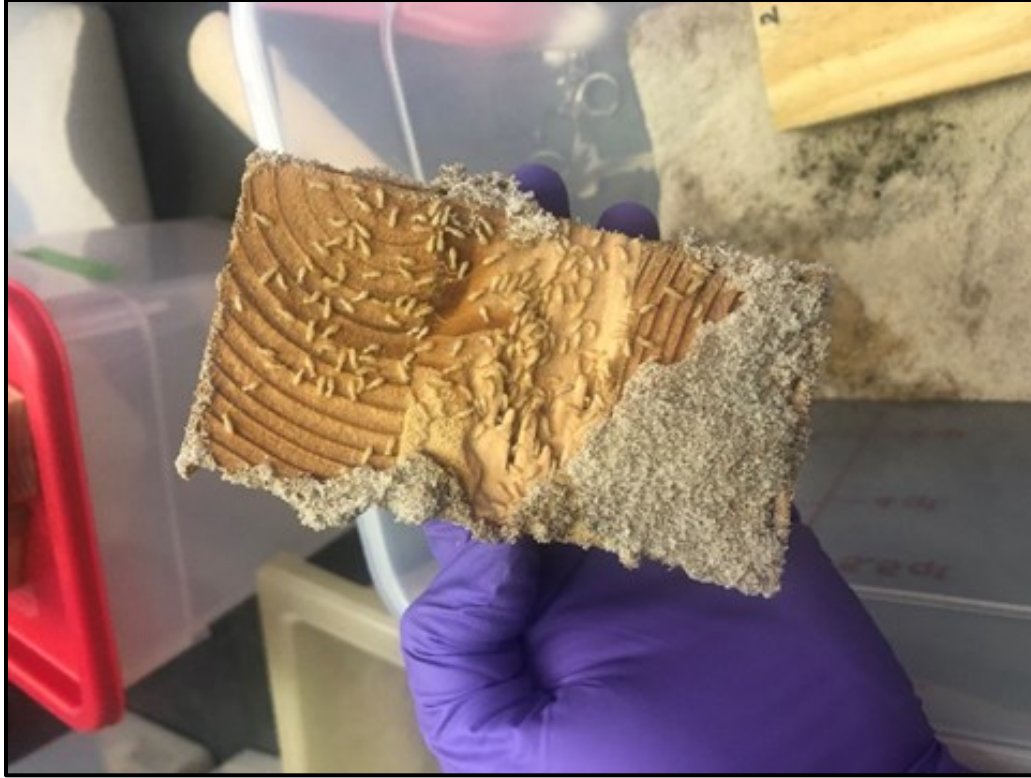
Figure 4.3 Presence of healthy and active termites when CLT is paired with solid SYP.
