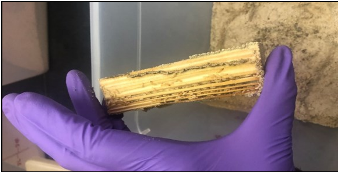
Figure 1.3 Active termite excavation along the springwood layers of growth rings.
